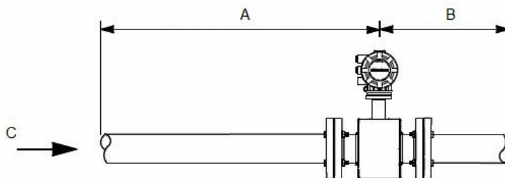
Figure 1: Upstream and downstream straight pipe diameters
