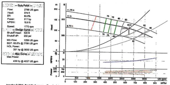
Impeller D-7513. Bowi Performance. To calculate pump performance refer to online catalog-Performance Calculations. Indicated Impeller diameter is average in accordance with the Hydraulic Institute Standards, pump is guaranteed for one set of conditions. Performance guarantees are based on shop test and when handling clear cold fresh water at see level and at a temp no greater than 85% %F. Suction
